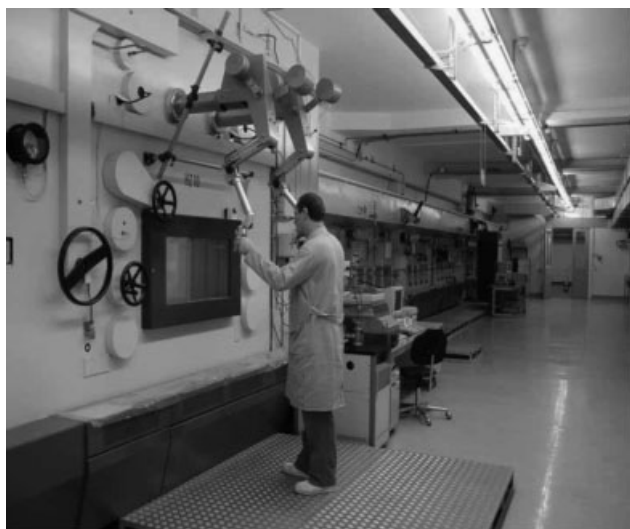
Figure 3 Operator's working place in front of a hot cell.
