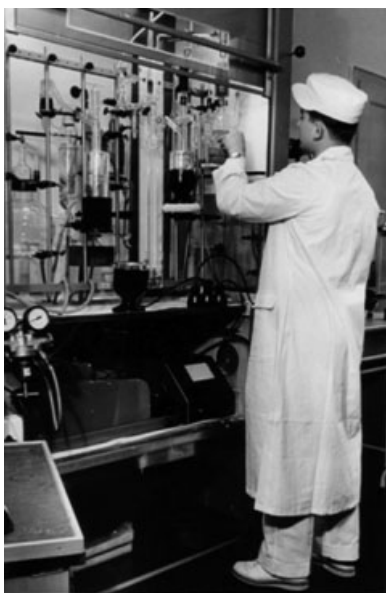
Figure 1 Synthesis of carbon-14-labelled organic compounds by means of vacuum line.
